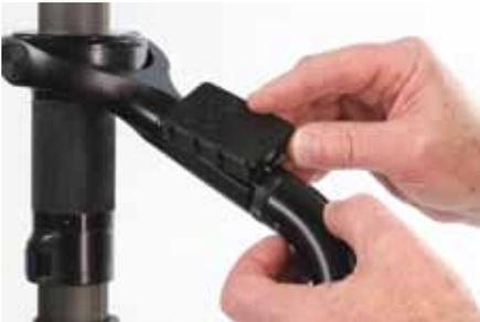
When returning the remote to the handle, insert the pins carefully and do not force anything.
