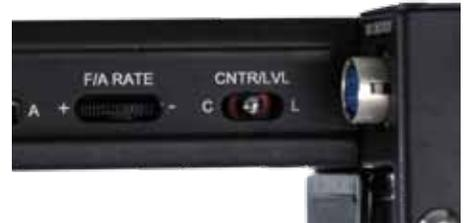
Pushing the double pole momentary switch on the “nosebox” to the “C” side centers the stage.
