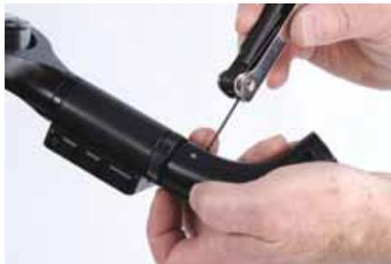
Orient the remote by screwing the curved handle in or out. If the handle is too far in, you can't easily remove the remote via the black knurled ring, and you might have to back the handle off one full turn. Loosening the setscrew a lot further and unscrewing the handle is also how you access the "tilt" bearings and shaft for cleaning.
