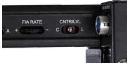
The center go-to button on remote shares the same preset as the “L” position on the switch on the nose box. The “L” position is programmed exactly like the center go-to button on the remote, and the red mode LED on the nosebox will flash to confirm programming.
