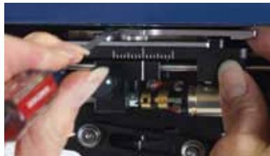
The stage is easy to adjust. The knob at the right rear controls fore-aft, and the two knobs on the side control side to side movement.
