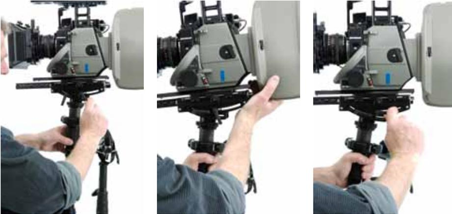
Note: Don't grab the stage by the nosebox to adjust tilt. Be sure to loosen the arc clamps fully and grab the camera or dovetail plate. Don't force anything; it should move fairly easily.
